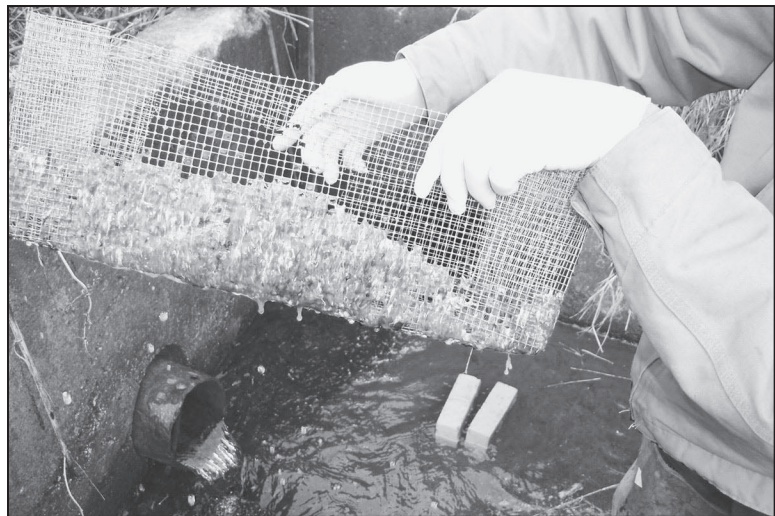
A visible example of untreated sewage being discharged, this photo shows the waste collected in one hour from tile line discharging into Clear Creek, south of Conroy, Iowa, January 2005. Photo courtesy D. Ratliff
