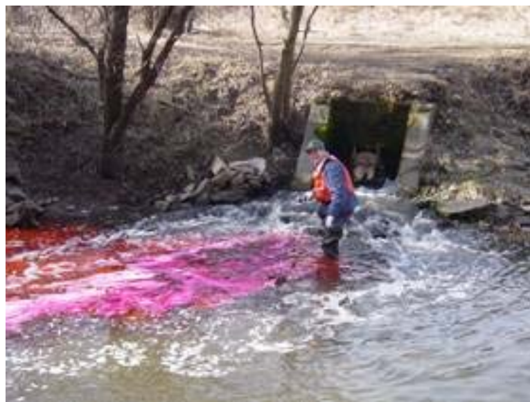
Figure 4A. Injection of dye at Fourmile Creek near Ankeny, Iowa at the wastewater treatment plant outfall, March, 2005.
