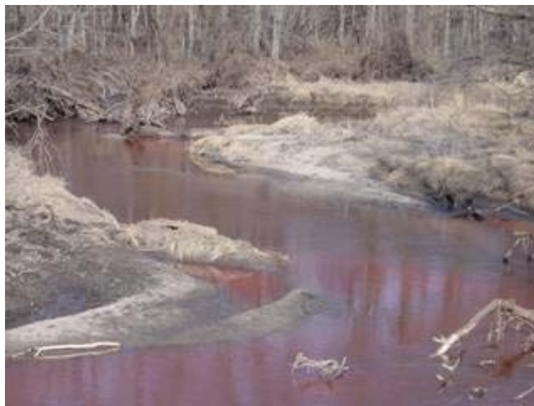
Figure 4D. Trailing edge of the dye concentration at Fourmile Creek near Ankeny, Iowa, site 3, March 2005.
